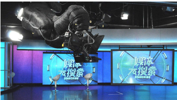
In combination with a linear track the robotic camera system can be used flexibly on all 8 different sets.
